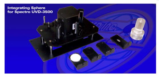
Integrating sphere is used to measure the diffuse reflectance of solid sample and powder, as well as measure the transmittance of the glass and membrane. Integrating sphere can analyze the chrominance, color difference, and whiteness.
