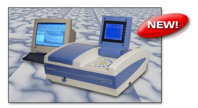
Spectro UV-2650 is a new single beam scanning UV-VIS Spectrophotometer; with its seamless integration with any PC, which makes managing data exceptionally easy. This spectrophotometer delivers enhanced ease-of-use, precision and accuracy resulting in time and cost savings, as well as unprecedented confidence in test results. Model UV-2650 works in the ultraviolet and visible range of 190-1100 nm and has a fixed bandwidth of 1 nm.
